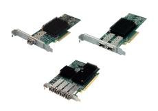
ATTO Celerity™ 32Gb Gen 6 Fibre Channel host bus adapters provide the highest performing SAN storage connectivity for physical and virtual infrastructures.
